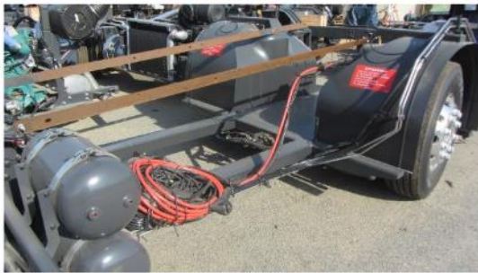
Low Coach Chassis with transport framing.
