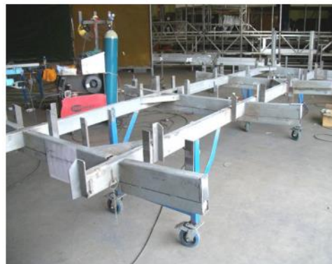
Chassis extension laser cut and jig made stainless steel.
