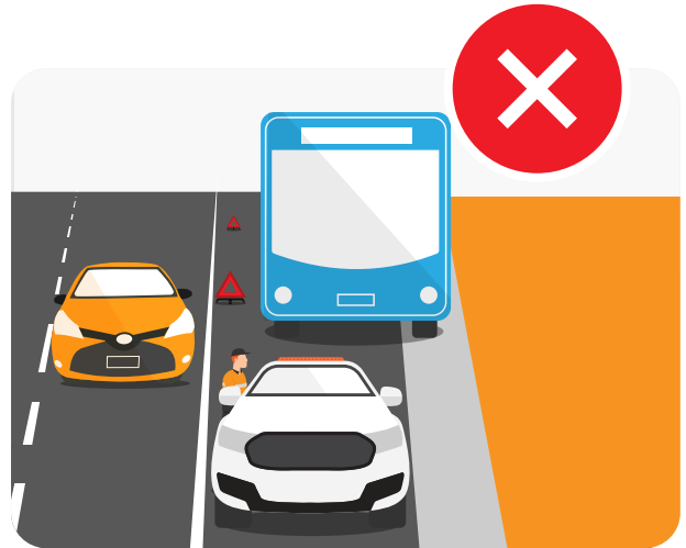
Only the rear of the repair vehicle is visible. Equipment stored on the right hand side cannot be safely accessed.
