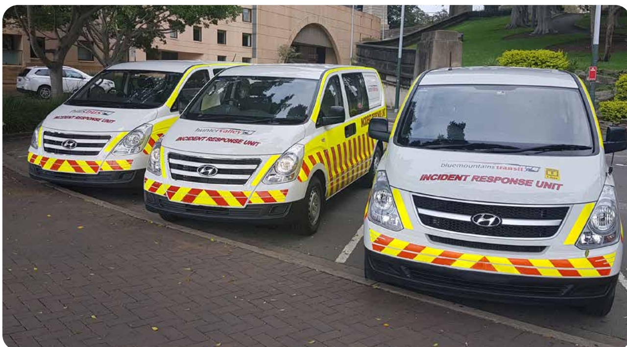
Hi Visibility and reflective markings provide additional safety for staff working in a dangerous environment.
