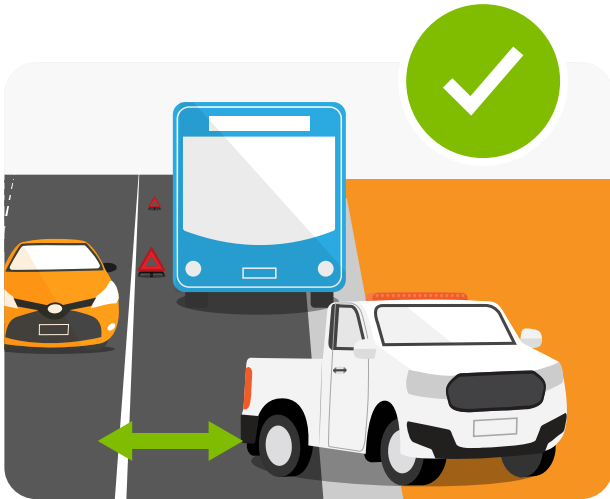
A 45 degree angle increases visibility for passing traffic.
